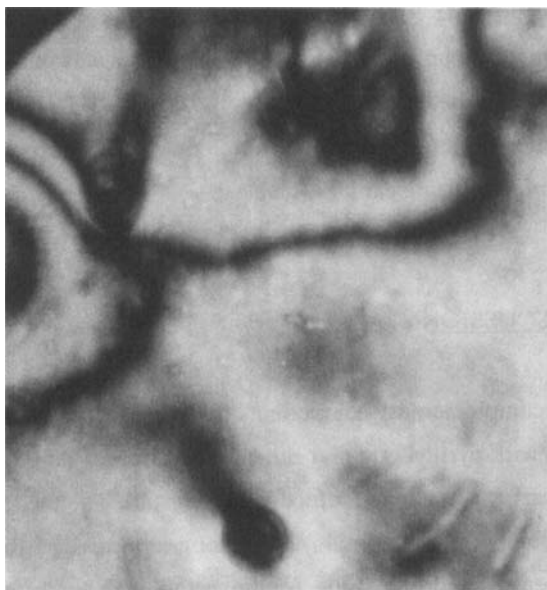
FIGURE 1 A typical nematic texture for the I-OC 5 B complex See Color Plate I.
